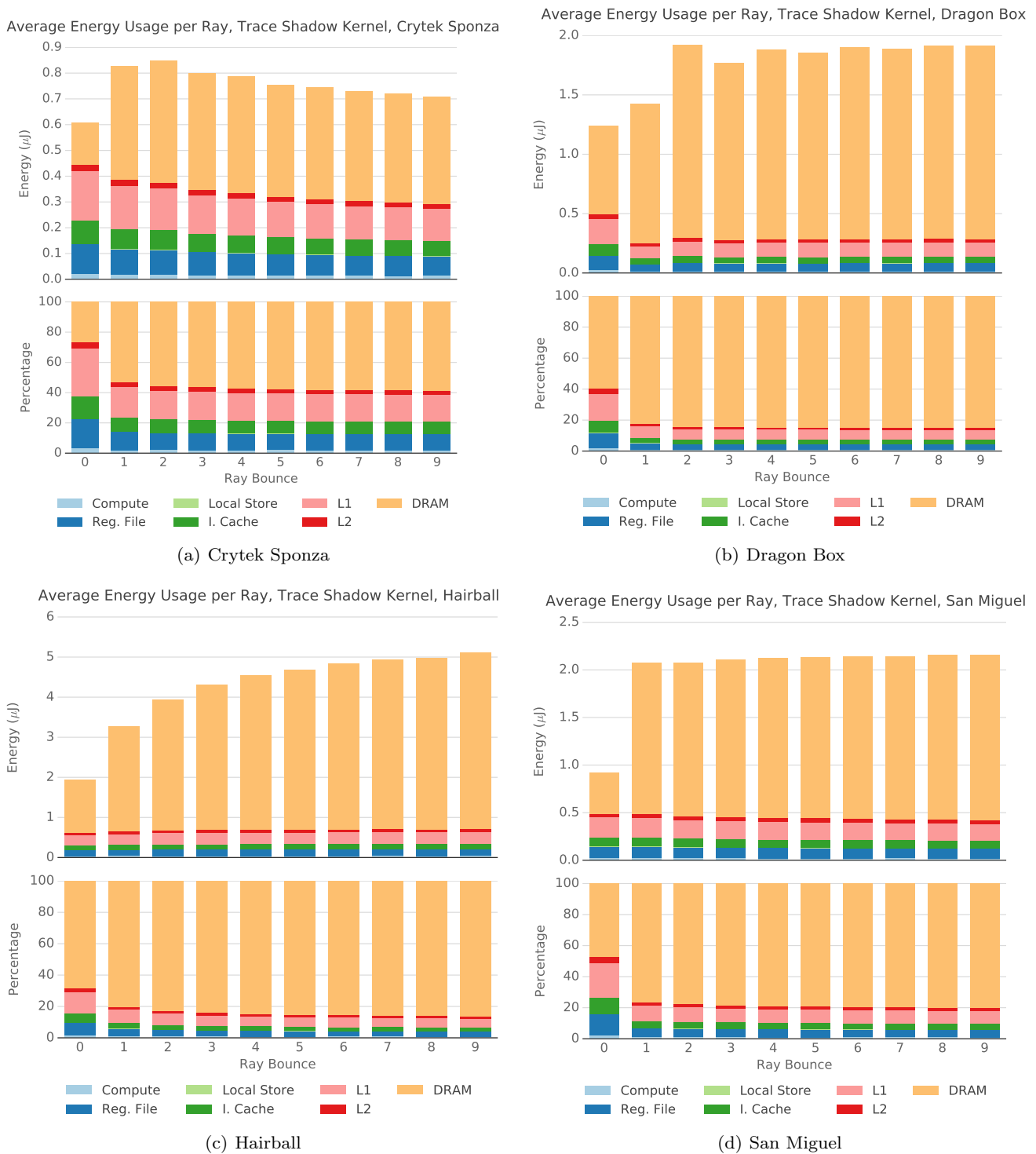
Fig. 12: Classification of energy contributions per ray by source for the Trace Shadow kernel. Each scene rendered with maximum of 9 ray bounces. Shadow Trace behavior is similar to non-Shadow Trace. Again, DRAM is taking up the majority of energy contribution. Memory usage in Hairball scene is most significant of all due to depth complexity.
